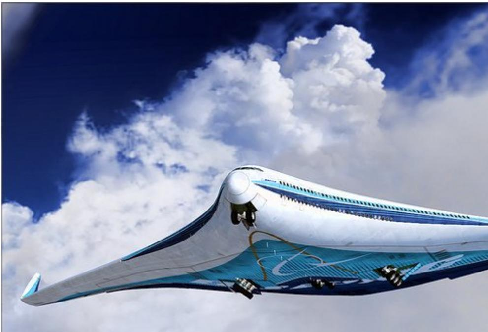
**There are several big advantages in the 'Blended Wing & Fuselage' design, the most important being the lift to drag ratio which is expected to increase by an amazing 50%, resulting in an overall weight reduction of the aircraft by 25%, making it an estimated 33% more fuel efficient than the A380, and thus making the Airbus's \$13 Billion Dollar investment look pretty shaky.**
